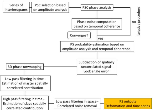
Fig. 2. Flow chart PSI processing in StaMPS method. (Modified from [5])
