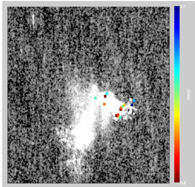
Fig. 8. Standard deviation of the estimated deformation rate.
